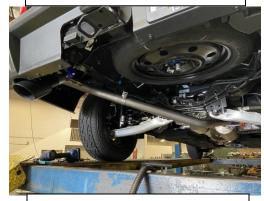
6. With proper clearance from spare tire, install the exhaust tip onto the tailpipe. The system was designed to have the tip 1" below the bumper panel of the vehicle. With the tip in your desired position begin to tighten down all clamp connections from the front head pipe back.
