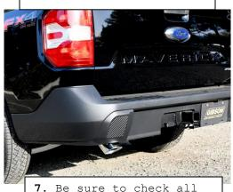
clearance after each section has been tightened to be sure there is proper clearance. It may take 4-500 miles for your vehicle to fully adjust to the changes in exhaust flow.
